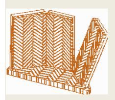
Step Two: (Allow 24 hours for base to cure.) Using Heat Stop Refractory Mortar; set the panels on the floor so the back of the panels align with the back of the floor. They are temporarily supported by concrete blocks or lumber.
