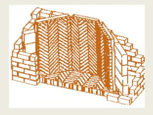
Step Three: A solid masonry backing wall at least 4 inches thick is built to permanently support the firebox. Cracks are filled with Heat Stop Refractory mortar and the washed with clean water. Continue with setting your throat, and treat like any other firebox, continue building fireplace and chimney.
