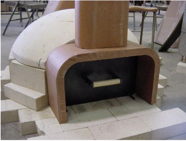
An oven "door" (free-standing steel screen) is provided to help keep the oven warm. When a fire is heating the oven the door can be placed toward the front of the entrance so that flue gasses can enter the flue. After the oven is warm and the fire is out the door can be placed farther in the entrance to close off the flue, seal the oven better and preserve the heat.
