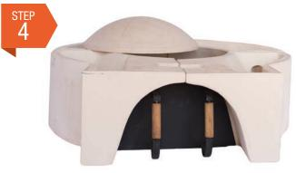
Set the oven dome on top of the base sections in HeatStop II refractory mortar.
